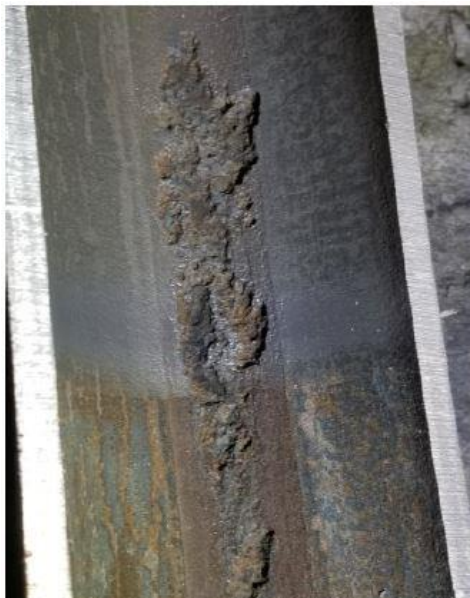
Untreated Joint 278 exhibiting some severe corrosion pitting
