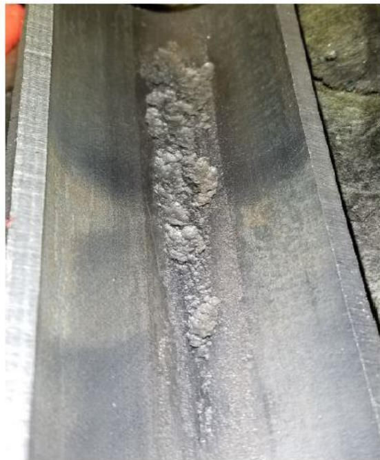
Untreated Joint 278 exhibiting some severe corrosion pitting
