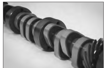
Fig. 2 — True contour hardening of camshaft lobes. Courtesy of Inductoheat Inc.
